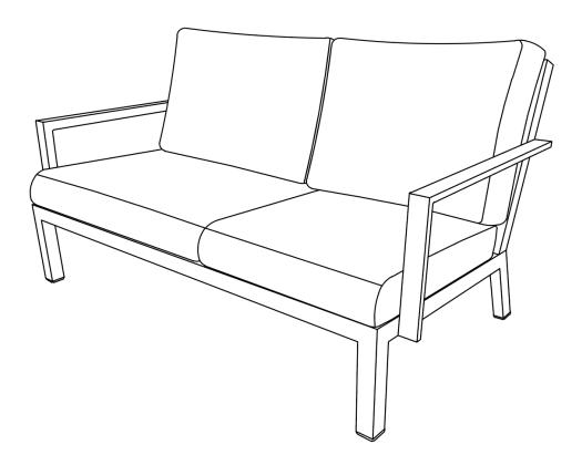
Insert all bolts and loosely finger tighten first. Once all bolts are in place, re-visit each bolt and fully tighten with the provided tool. Do not fully tighten bolts one by one.
